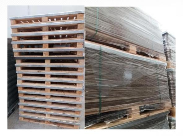
Cardboard and plastic sheets, since packaging is particularly vulnerable to damage during storage and transport, should be placed on a pallet per 500 pieces. They must be secured from above and covered with a foil. Each pallet with intermediate boards shall also be strapped and shrink wrapped, to avoid damage to the shipment during transport. The intermediate board should not be more than 1.5-1.5 cm larger than the pallet.
