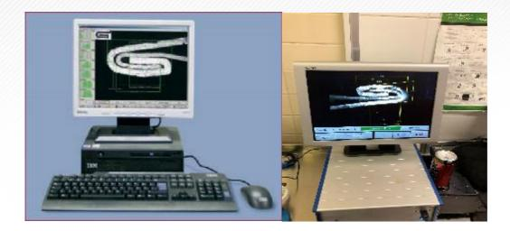
The software allows you to perform various calculations to fully measure the seam. This measurement method is the industry standard for measuring and analysing the seam and is the only method by which we get a response to the size of the critical parameter, the seam gap.
