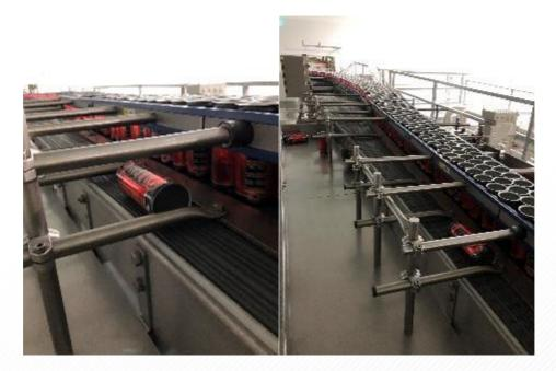
When choosing material for the conveyor, copper and brass should be avoided due to corrosion. It is advisable to cover all surfaces with hard plastic, which protects the cans from damage, and facilitates the progress of the cans on the conveyor. This is true for turner guide as well (see photo). Turner
