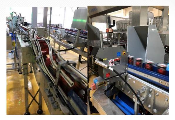
Where conveyor belt sensors are used, the sensors shall be motion sensors and not pressure sensors. They shall be placed in such a way as to avoid any damage to the cans. Conveyor management is designed to ensure that the effect (pressure) that cans put on each other is only of the necessary extent, and the belts do not move under the cans unnecessarily. Antistatic materials shall be used.
