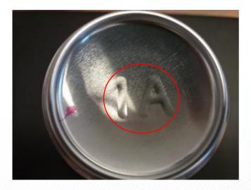
**Dotted code** Serial number of the can machine tool (e.g. 10)
