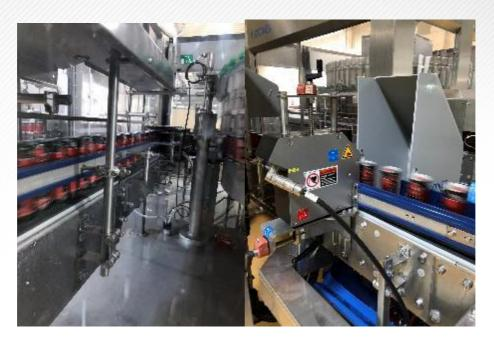
In order to allow the overturned cans to leave the conveyor and avoid their damaging the other cans, the gap between the side guides should be big enough for the cans to be able to fall out (see photo). It is recommended to equip such places with a can collecting tray.
