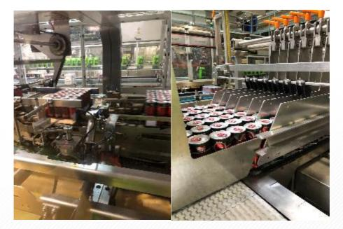
Conveyor management shall be designed and set so that the belts do not move under the standing cans.
