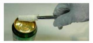
4. Place the cotton wool in the leakproof containers and immediately weigh it again (the least possible time should go by between sampling and measurement). Record the results.
